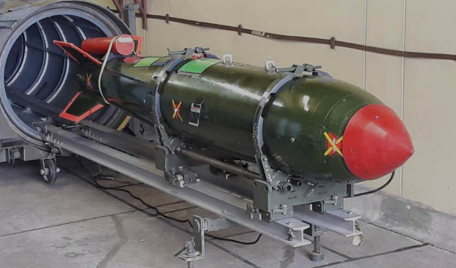
A WE177 A training round - an inert ballistic casing used for ground crew instruction in weapon handling and loading.
