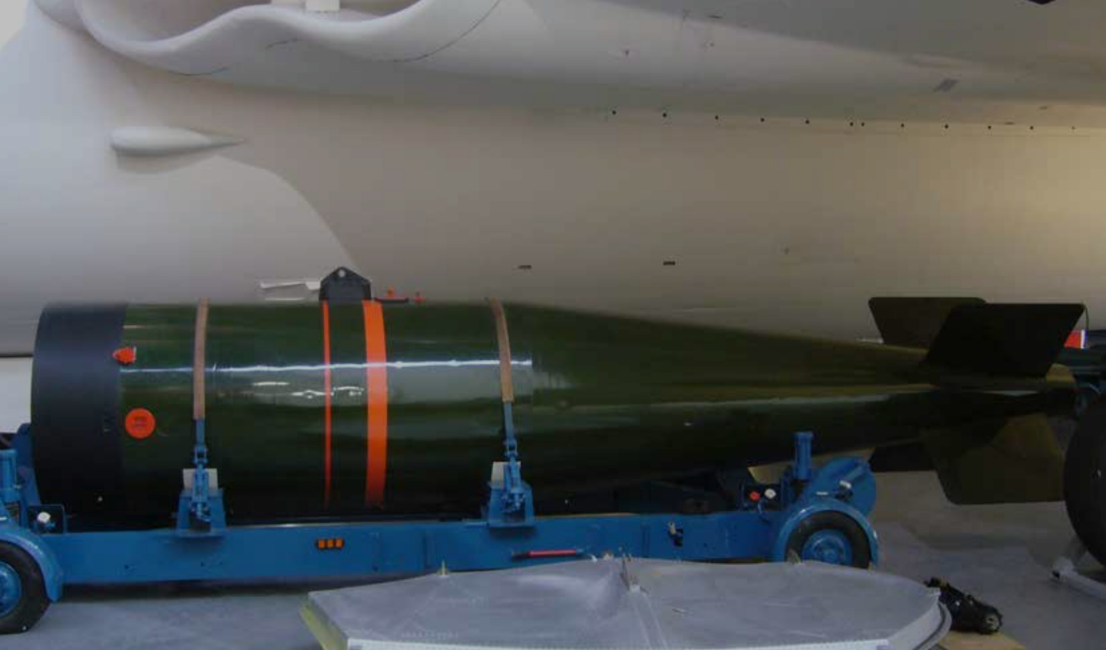
A Yellow Sun Mark II ballistic casing carrying the Red Snow one megaton warhead. Photo taken by Tom Oates, 2011.
