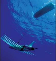
Wave Glider with powerful sensors, and with surface board providing continuous power and communications
