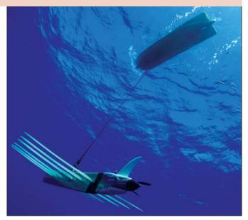
Wave Glider drone from below, packed with extremely sensitive sensors with long range reach
