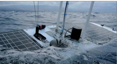
Wave Glider surf board with solar power and communications, attached to drone below the surface
