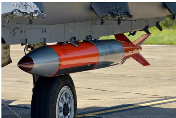
Prototype inert B61-12 fitted to a US Air Force F15-E
