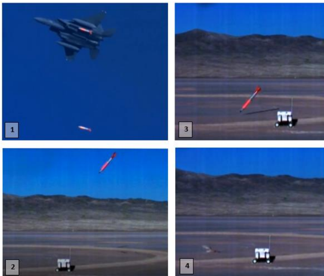
A US Air Force F-15E drops an inert B61-12 during testing in October 2015. Official images from the test indicate that the B61-12 demonstrated accuracy of less than 30 metres and that the guided bomb has earth-penetrating capability that could be used against underground and hardened targets.
